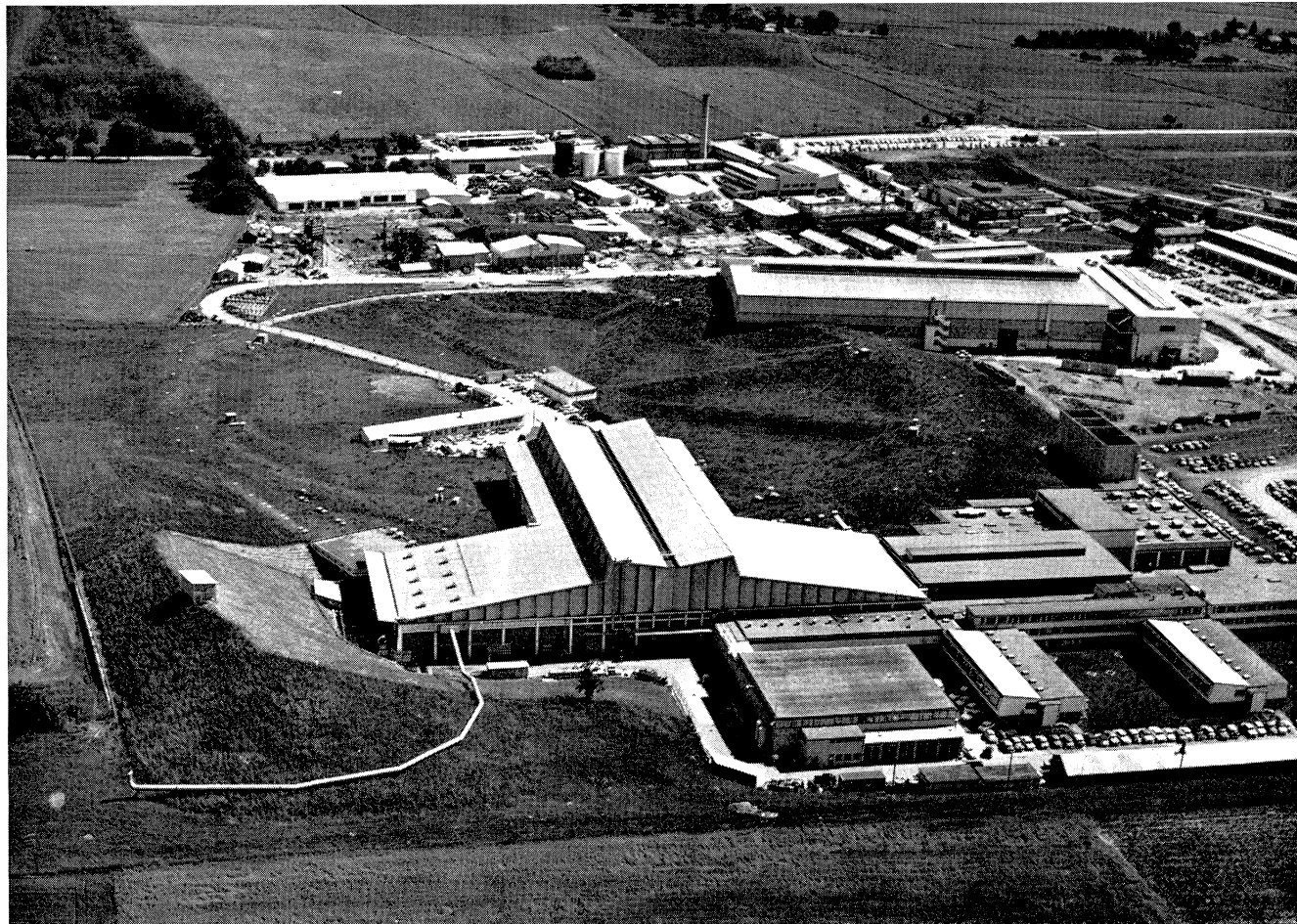
The proton synchrotron at CERN, which accelerates protons to an energy of 28 thousand million electronvolts, for investigating the structure and properties of fundamental particles. Looking rather like a giant cartwheel partially buried under the earth, this machine has a mean diameter of 200 metres. In the centre foreground are the North and South experimental halls, with the adjoining laboratories, offices, and equipment buildings ; on the other side of the ring the East experimental hall leads off tangentially to the bubble-chamber building. Other CERN buildings can be seen in the background.
